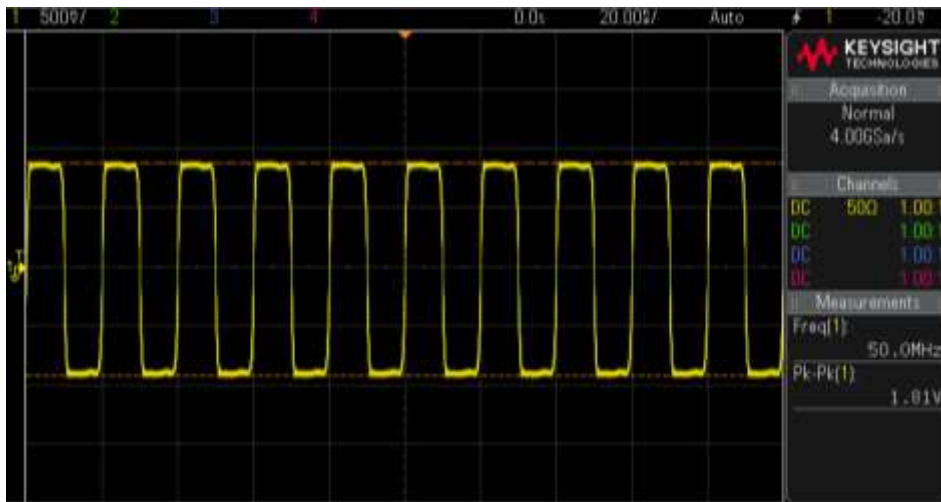
The outputted 50MHz 2Vp-p square waveform.
